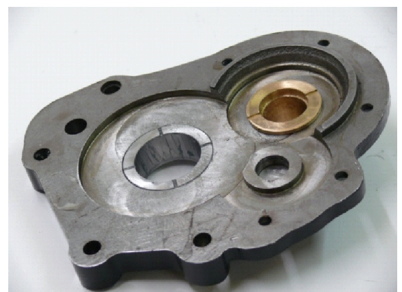
Image below shows the sidecover necessary to hold the 4-Speed gears. Sold separate from the conversion set, comes with a complete Gearbox
